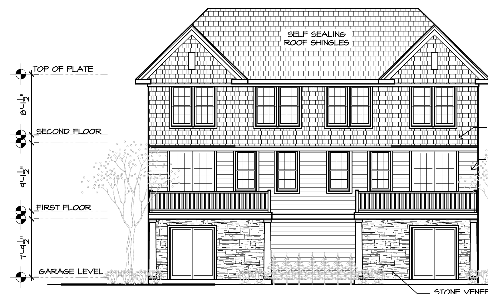
REAR ELEVATION BUILDINGS 3, 8 & 5 - TYPES C & D
