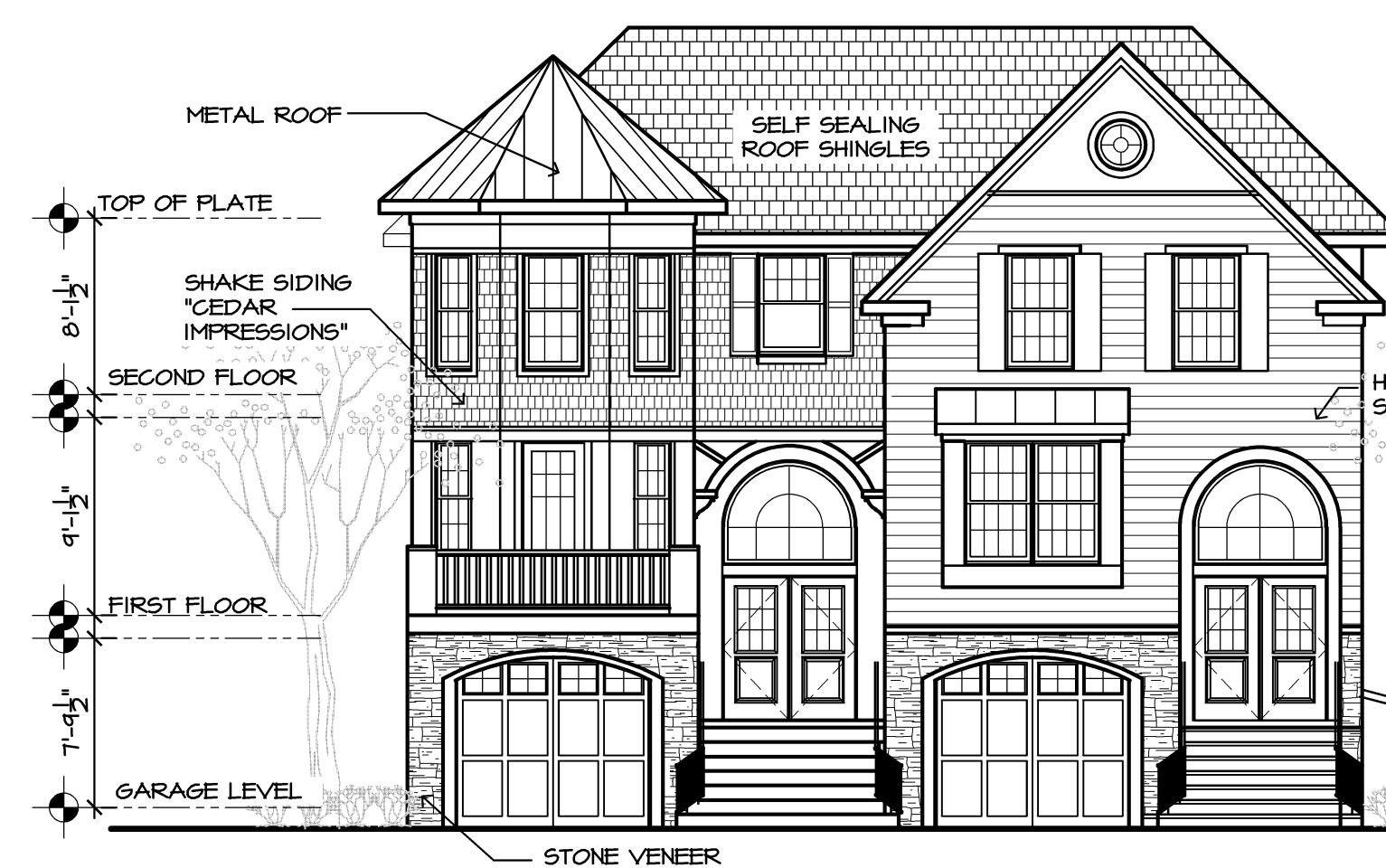
FRONT ELEVATION BUILDINGS 4 & 6 - TYPE A
