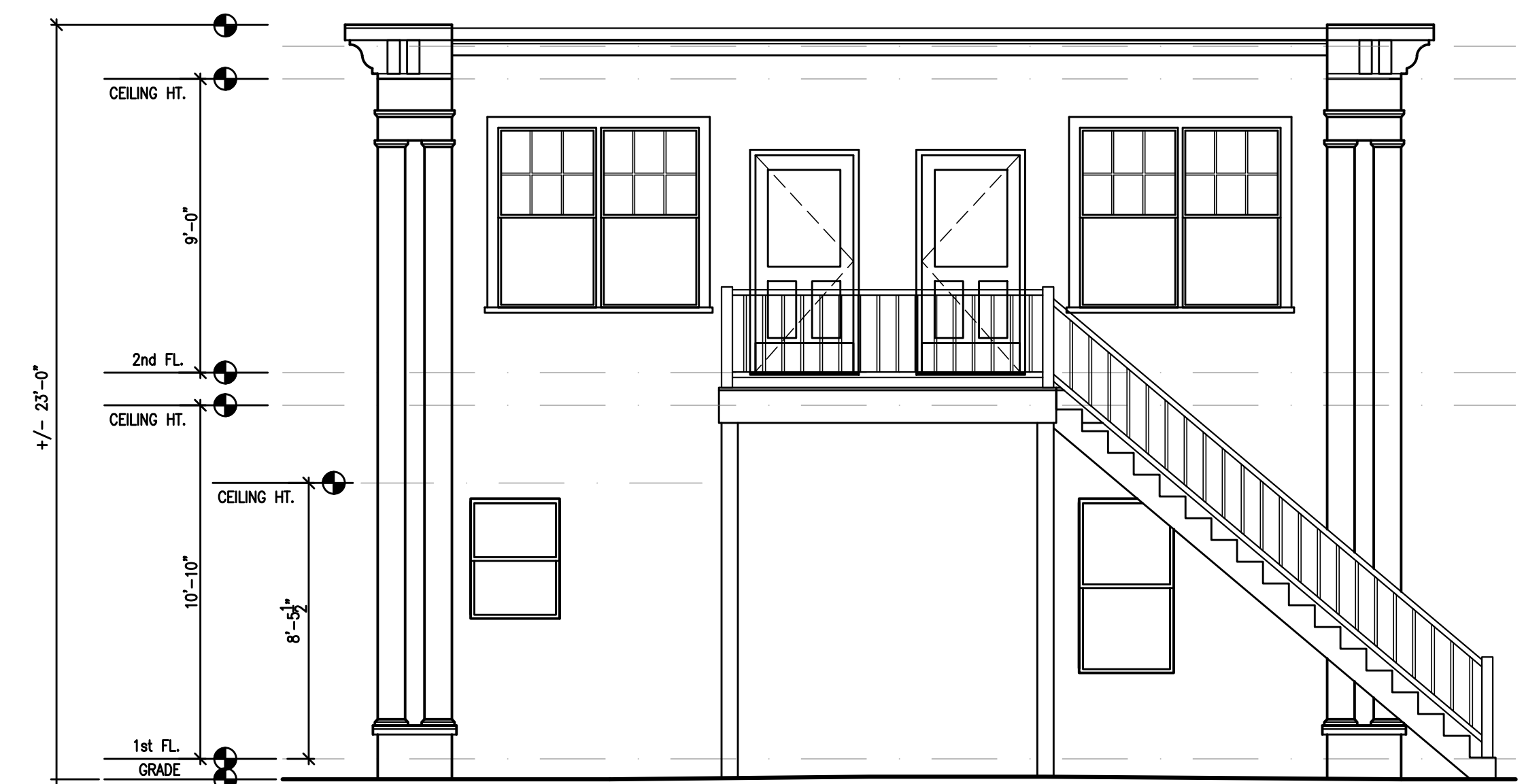
○ REAR ELEVATION Scale: 1/4"=1'-0"
