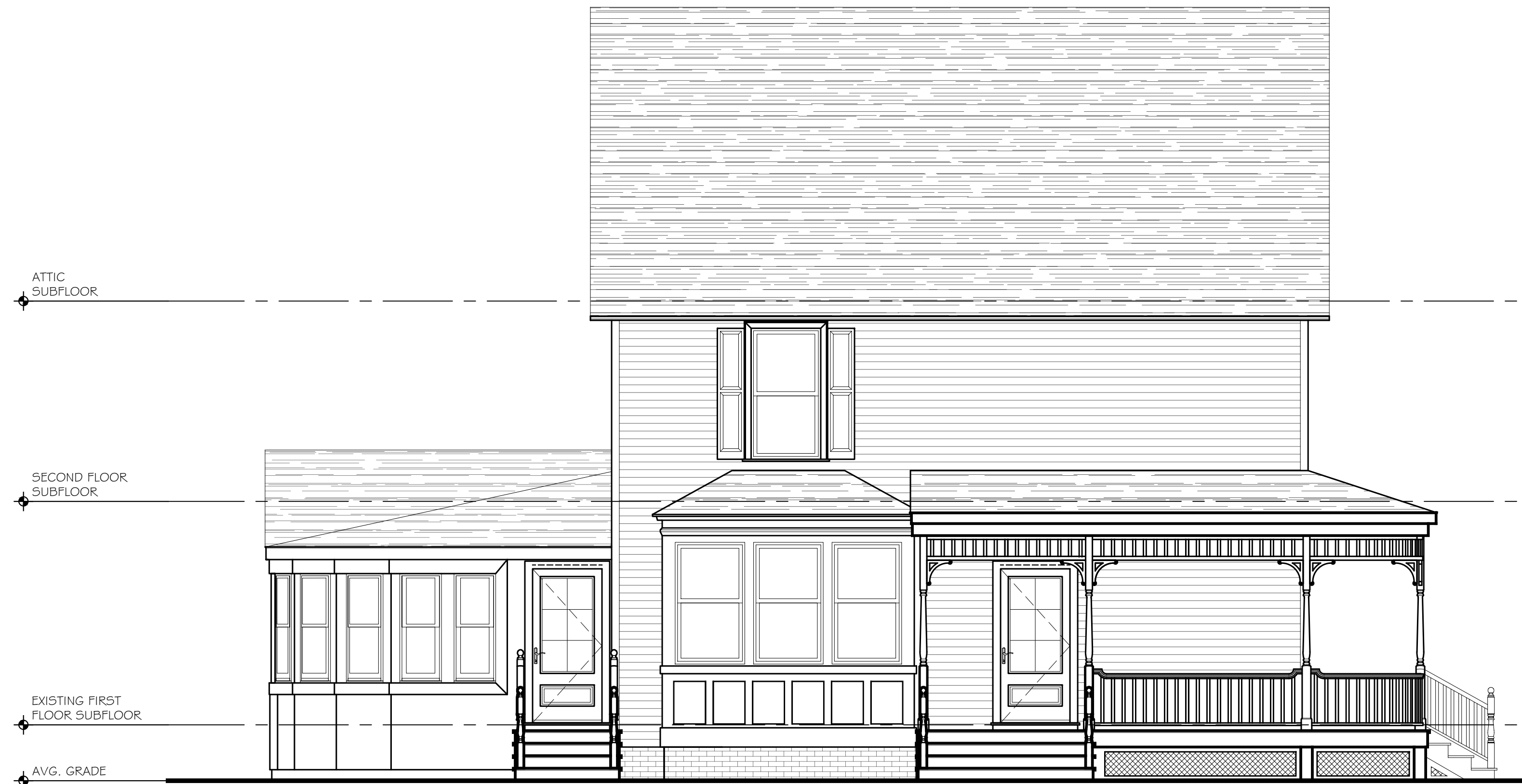
4 LEFT SIDE ELEVATION SCALE: 1/4" = 1'-0"
