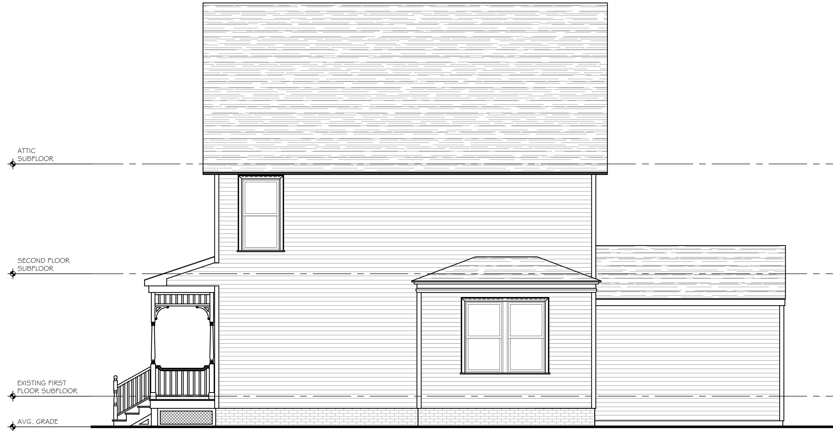
2 RIGHT SIDE ELEVATION SCALE: 1/4" = 1'-0"
