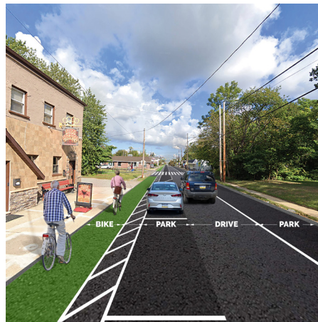
Protected bike lane
