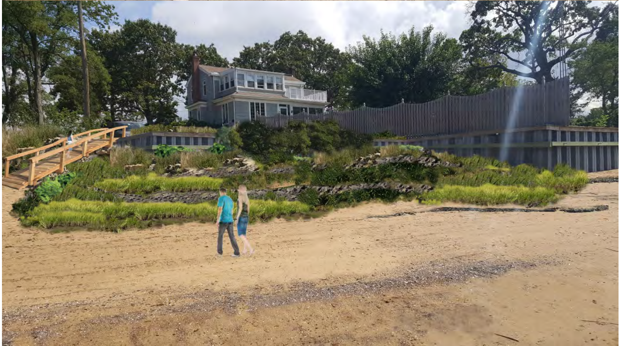
Figure 193: Existing bulkhead at Walnut Street street-end (top) and rendering of a new bulkhead with ecologically enhanced revetment where there is existing bulkhead (bottom) (Source: Maser Consulting, P.A.)
