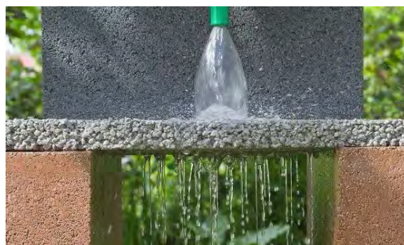
Figure 236: Example of water draining through permeable pavement 144
