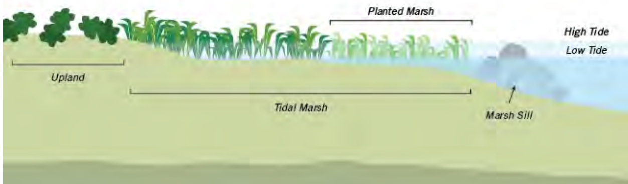
Figure 185: Diagram of a marsh sill in a tidal marsh (Source: The Nature Conservancy)
