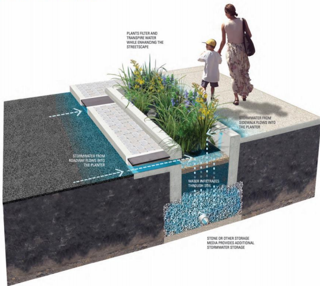
Figure 2.1: Three-Dimensional View of a Stormwater Planter
