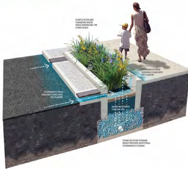
Figure 2.1: Three-Dimensional View of a Stormwater Planter
